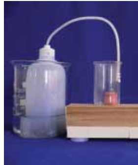
Fig 9: Apparatus to produce hydrogen sulphide gas
