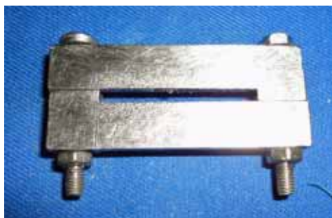
Fig. 1 Split Stainless Steel mould used to fabricate the bar specimens for flexural strength
