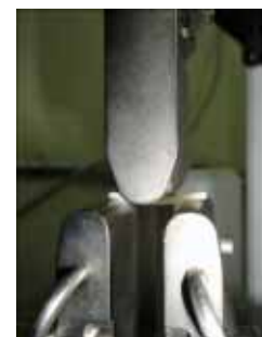
Fig. 3 Flexural test under progress.
