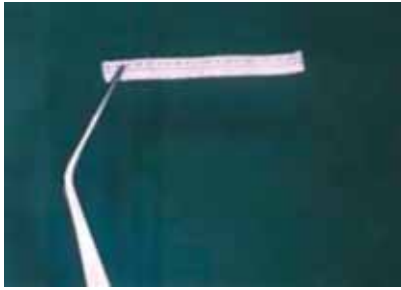
Fig. 3 Ribbon fiber cut to measurement ready for placement.
